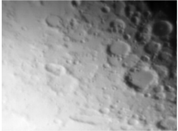
Figure 4. Images of the day side lunar surface. The 11.6 \mu\text{m} image has a FOV of 7x5 arcmin and an effective resolution of 3.4 arcsec.
