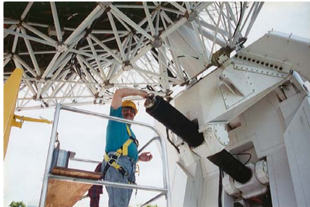
Figure 1: Left, the SMA antenna mount, made of 130 mm thick steel plate to meet the antenna stiffness requirements for pointing. Above, detail of the interface between the antenna pedestal and the reflector assembly. Note the ball-screw drive and the four flex-pivots used to connect the carbon fiber central hub of the reflector assembly to the steel weldment that connects to the elevation axis and screw drive.
