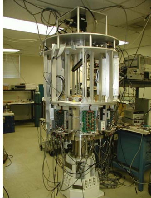
Figure 6: Left, schematic of the SMA receiver system showing the optics, receiver insert, and cryostat assemblies. Right, photograph of a complete SMA receiver system showing the cryostat surrounded by the receiver control electronics, the optics cage supporting the various sets of receiver coupling optics, and the central wire grid assembly used to select between the lower frequency receivers. The near-field scanning unit is also visible in place of M6 at the center and above the complete receiver system.
