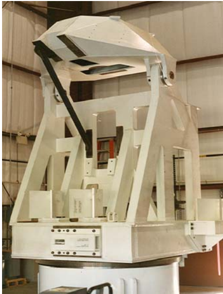
Figure 1: Left, the SMA antenna mount, made of 130 mm thick steel plate to meet the antenna stiffness requirements for pointing. Above, detail of the interface between the antenna pedestal and the reflector assembly. Note the ball-screw drive and the four flex-pivots used to connect the carbon fiber central hub of the reflector assembly to the steel weldment that connects to the elevation axis and screw drive.
