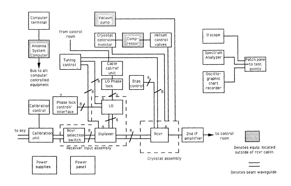
Block Diagram for Receiver Cabin Electronics
