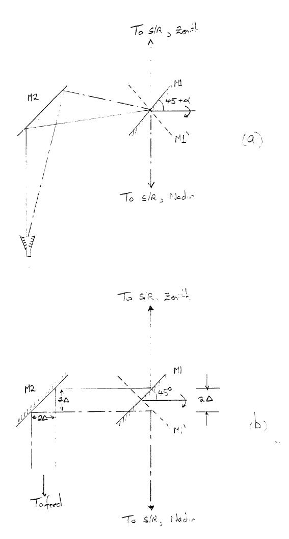
Figure 8: Suggestion for accessing a Coude focus with the same two transfer mirrors required to feed the Nasmyth focus.
