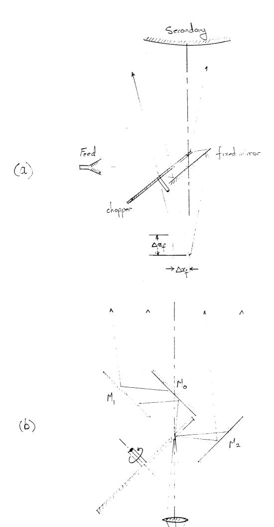
Figure 10: Sketch of basic optics of an aperture plane wobbler (intended to move the final beam on the sky).
