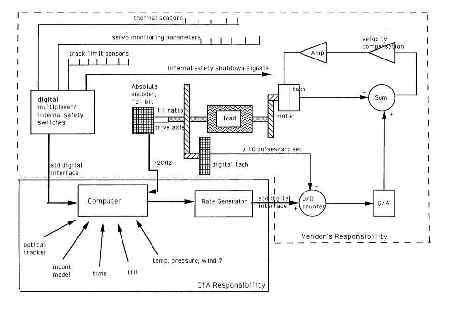
Figure 2: Schematic Representation of a one axis control system
