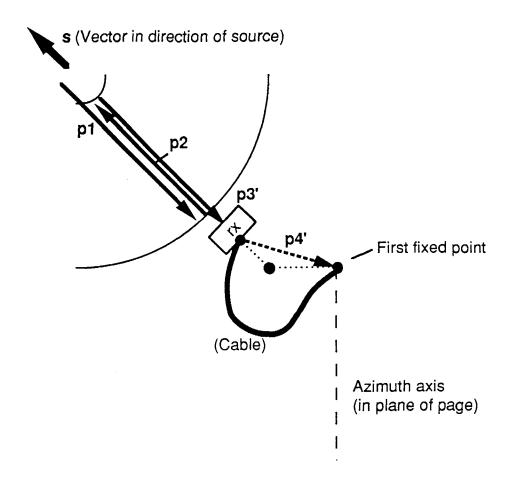
Figure 2. Optical paths in an alt-az antenna with non-intersecting axes and a Cassegrain receiver. **p4'** is the vector for the path which is actually traversed by the cable. The thin dotted lines show that **p4'** can be broken up into one part parallel to **s** and one part equal to the vector **p4** in Figure 1.
