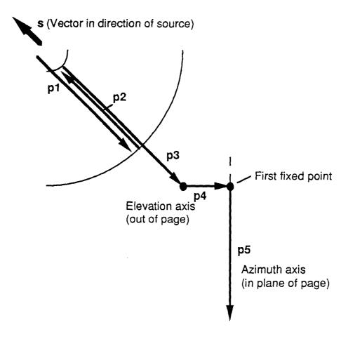
Figure 1. Optical paths in an alt-az antenna with non-intersecting axes.
