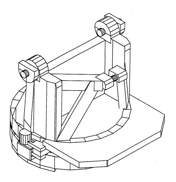
Figure 2 - SMA Mount Model with 2.7 meter azimuth bearing
