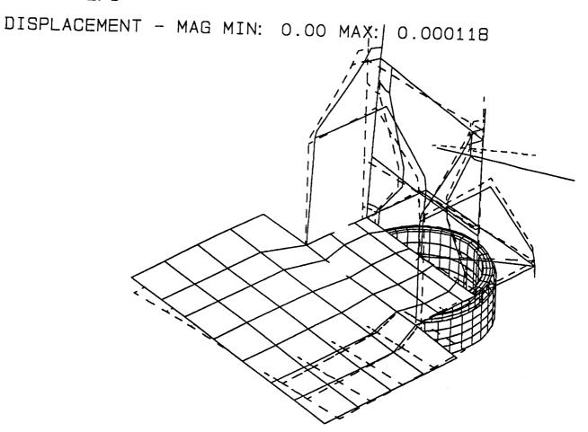
Figure 8 - Mount Deformed Geometry - Wind Case 2
