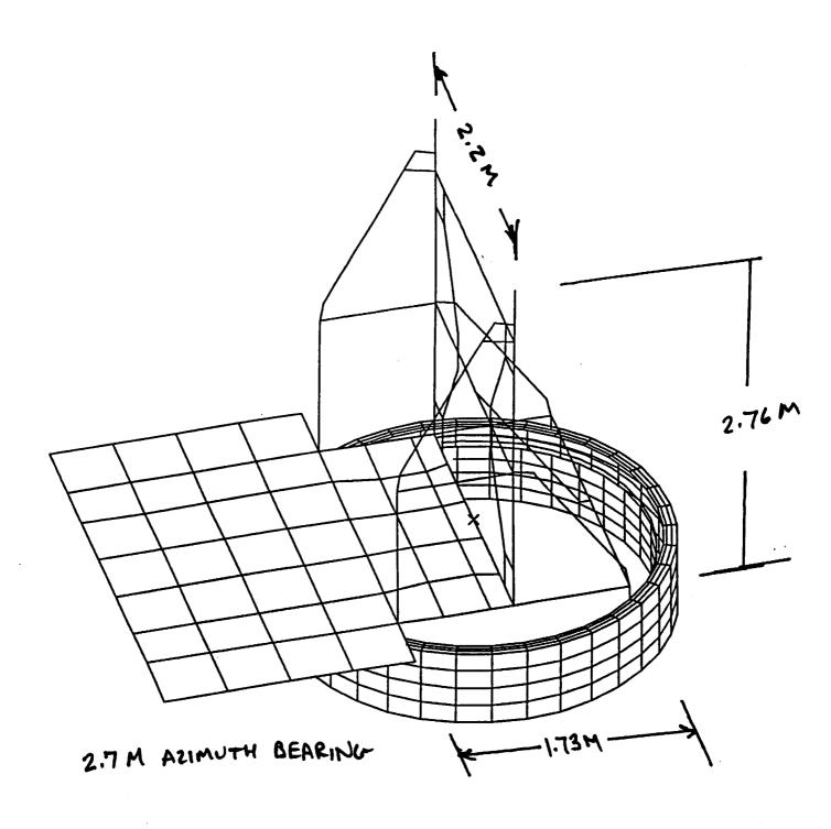
Figure 3 - SMA Mount Model with 1.6 meter azimuth bearing
