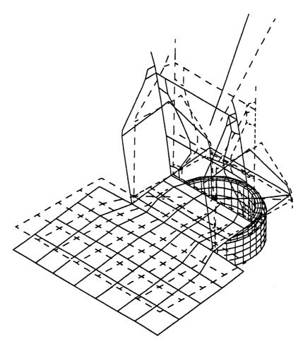
Figure 10 - Mount Deformed Geometry - Wind Case 4
