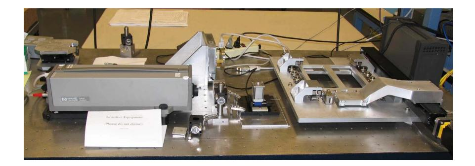
Measurement of Mechanism Positioning Precision and Repeatability with a Laser Interferometer
