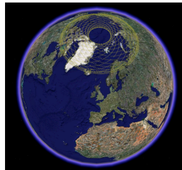
FIGURE 2. Measurement locations for SOFIE. Yellow dots indicate tangent point locations for a six-month period (Jun – Dec, 2007). The tangent point latitude oscillates slowly between 65 deg N at solstice and 85 deg N at equinox. A similar pattern develops in the Southern hemisphere (not shown).
