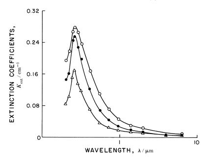
Figure 4. Measured spectral extinction coefficients for the premixed propane-oxygen flame with  $\phi = 1.8$ .  $H \text{ (mm)}: \Delta, 6; \bullet, 10; \circ, 16$ .
