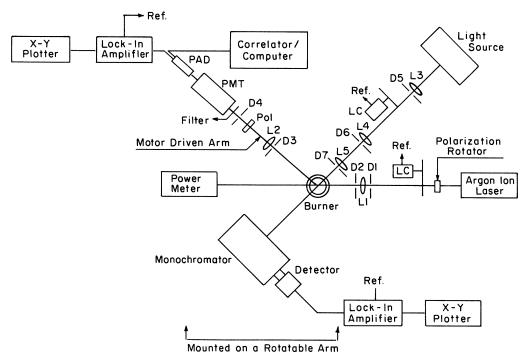
Figure 1. Plan view of the light scattering system.
