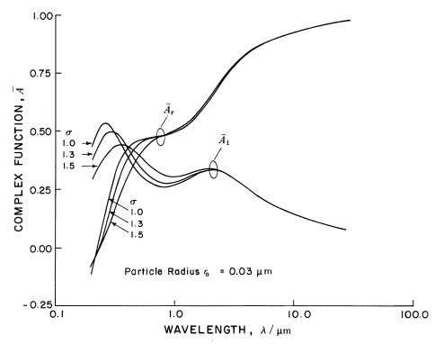
Figure 3. Variation of the functions  $\bar{A}_i$  and  $\bar{A}_r$  with respect to geometric width ( $\sigma$ ) and wavelength ( $\lambda$ ). The particle radius used was 0.03 µm.
