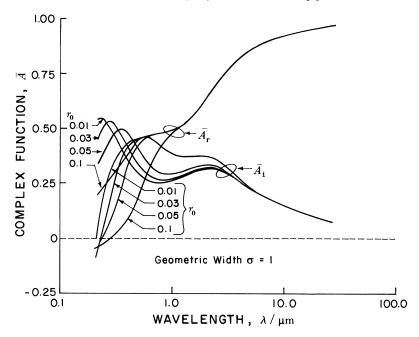
Figure 2. Variation of the functions  $\bar{A}_i$  and  $\bar{A}_r$  with respect to the wavelength for particle radii in the range 0.01 to 0.1 µm.
