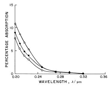
Figure 6. Percentage absorption measurements for a non-sooting propane-oxygen flame from 0.2 to 0.35  $\mu$ m. H (mm):  $\triangle$ , 6;  $\bullet$ , 12;  $\bigcirc$ , 16.
