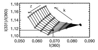
**Figure 1.** Ratio of the top of atmosphere radiances at 331/360 nm as function of 360 nm radiance for fixed value of aerosol optical depth. The solid circle represents the retrieval of  $k_{360}$  and Z associated with a hypothetical set of satellite measurements. The aerosol layer height and imaginary part of refractive index increase in the direction of the arrows.
