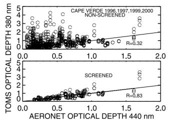
**Figure 3.** Comparison between TOMS optical depth retrievals and AERONET measurements. Solid lines represent the one-to-one relationship between two optical depths. R is the correlation coefficient between two data sets
