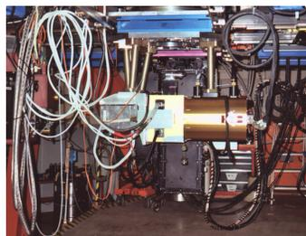
MIRSI on the IRTF. MIRSI was designed to look upward when attached to the IRTF's Cassegrain focus in order to eliminate intermediate, warm optics from the optical path.
