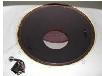
2. Remove the f/5 wavefront sensor.
