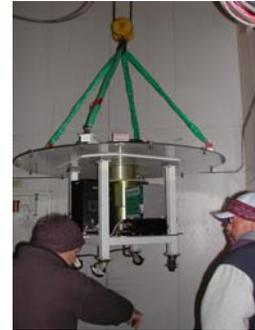
Alternatively, the large interface plate can be un-bolted from the instrument cart and each piece rolled into the elevator. However, the interface plate must remain electrically isolated from the cart when it is re-attached to the instrument cart; check this with an ohm meter before mounting the instrument to the telescope!
