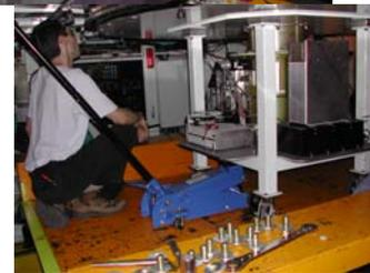
d. Use guide pins to align the bolt holes to the mounting flange.
