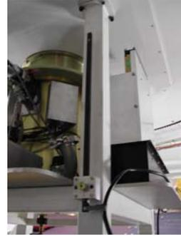
i. Connect the orange fiber to the Megacam Science EDT plug and to the white box on the back of the SWIRC electronics box. Tie the fiber spool down as shown.
