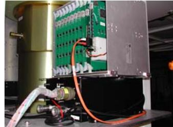
ii. Connect an Ethernet cable to the black Intelligent Instrumentations EDAS box.
