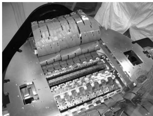
Figure 4. Flex circuits inside the cryostat. In this photo, one of the outer rows of CCDs is already installed and connected. Zener diodes are soldered onto the flex circuit to provide ESD protection.
