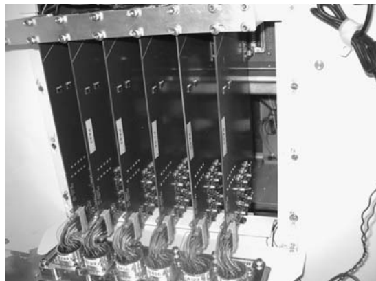
Figure 3. Preamp cards. The upper end of each card connects to the electronics rack backplane. The bottom end connects to the hermetic connectors. Each preamp card serves 3 CCDs.
