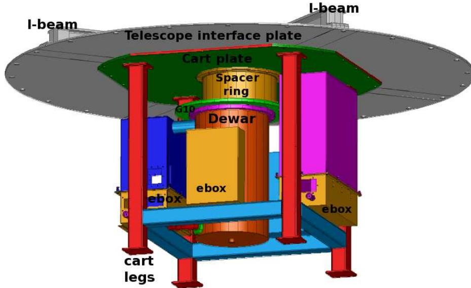
Figure 4. SWIRC instrument cart and telescope interface plate.
