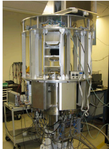
Above: Left: SMA cryostat with 600 GHz receiver insert, LO unit, and coupling optics in the lab in Cambridge, MA. Right: Observations of 658 GHz water maser line toward VX Sgr. Spectrum is a vector average of all baselines containing Antenna 2 (with upgraded 660 GHz receiver insert).
