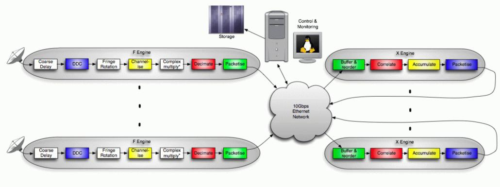
\*Complex multiply allows for fine delay control and per-channel digital gain control. White coloured blocks not yet implemented.
