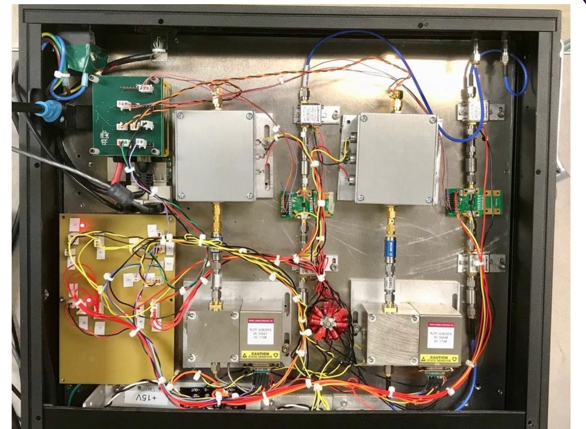
Above: The prototype Scanning Spectrometer system developed to measure the system temperature and gain of the wideband front-end receiver as a function of IF frequency. This information will be used to weight the different frequency channels when forming continuum images from wSMA data, as well as for diagnostic purposes when setting up the receiver systems. The two IF signals from the front-end receiver enter on the top right, are amplified and gain controlled before being filtered by YIG tunable filters and then detected by diode power detectors. The Raspberry Pi with its daughter boards on the top right samples the detector outputs and provides the control signals to sweep the YIG filters. The sampled spectra are then sent to the SMA control system via Redis over the SMA network.
