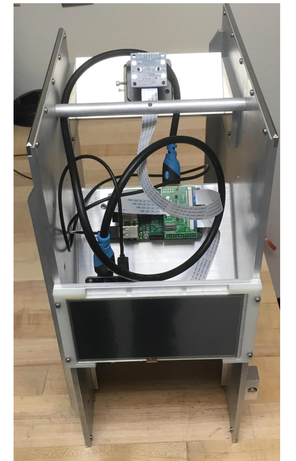
Above: A Raspberry Pi (lower right) with attached camera has been installed on the SMA to monitor the position of the waveplates in the Waveplate/Cal Load assembly. This camera allows the angular scale on the waveplate mounting hardware to be read while characterizing the instrumental polarization of the SMA during dual-polarization testing.
