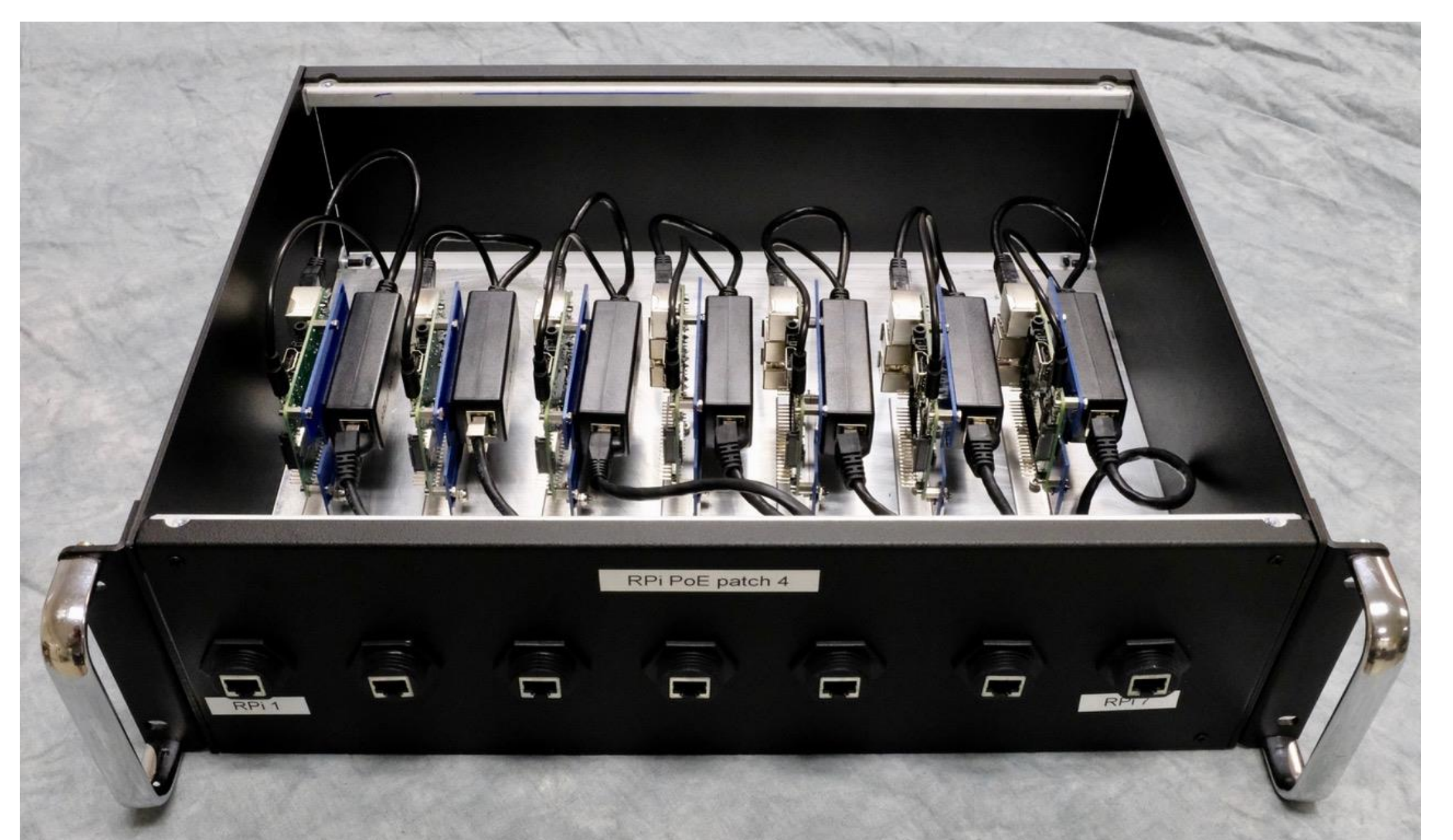
The most recent version of the Raspberry Pi Patch. This features 7 Pis with separate external Power over Ethernet (PoE) splitters and power supplies. Each Pi will be connected to a PoE switch that provides both Ethernet connectivity and power to the Pi, which can be switched on and off by the PoE switch.
