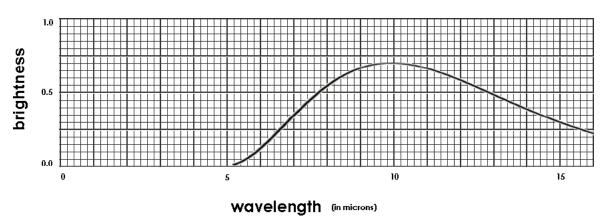
**Interpretation:** This shows the light emitted by the planet in the mid-infrared range. It is the "blackbody" curve that all objects emit, and that is characteristic of their temperature. The curve peaks at a wavelength of about 10 microns. This corresponds to a temperature of about (2900 / 10) = 290 degrees Kelvin, or about 17 degrees Centigrade = 63 degrees Fahrenheit. Not a bad average temperature for a planet.
