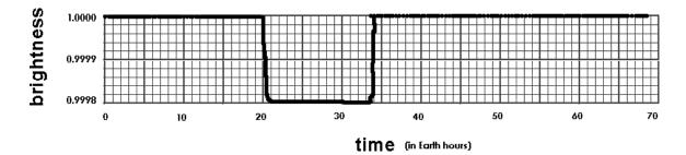
**Size of planet:** This planet blocks out 0.0002 of the star's light when it transits. For comparison, the Earth would block out 0.0001 of a sun-like star's light (since the Earth is 0.01 times the diameter of a sun-like star and we have to square this to compare the area of their disks.) So the mystery planet is a little bigger than Earth. You would presumably weigh more on this planet, but we don't yet know what it is made of, so we don't know its mass or gravity.
