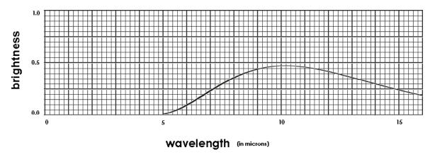
**Interpretation:** This is (infrared) light that is *emitted* by the planet itself. The peak in the curve—the wavelength where the most infrared is emitted—is at about 10.1 microns. This peak is determined by the temperature of the planet:
