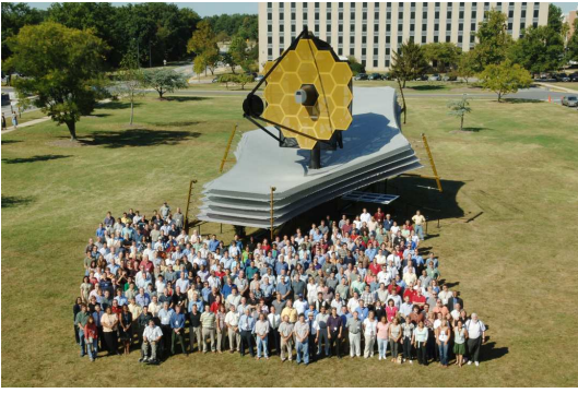
Figure 5: A full scale model of the James Webb Space Telescope (JWST), the successor to the Hubble Space Telescope. JWST includes a primary mirror 6.5 meters in diameter, and offers instrument sensitivity across the infrared wavelength range of 0.6\text{--}28\mu\text{m} which will allow detection of the first galaxies. The size of the Sun shield (the large flat screen in the image) is 22 meters \times 10 meters (72 ft \times 29 ft). The telescope will orbit 1.5 million kilometers from Earth at the Lagrange L2 point. Image credit: JWST/NASA ( http://www.jwst.nasa.gov/ ).
