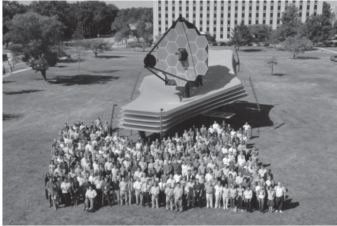
Figure 10.2 A full-scale model of the James Webb Space Telescope (JWST), the successor to the Hubble Space Telescope ( http://www.jwst.nasa.gov/ ; see Color Plate 19 for a color version of this image). JWST includes a primary mirror 6.5 m in diameter and offers instrument sensitivity across the IR wavelength range of 0.6 to 28\ \mu\text{m} , which will allow detection of the first generations of galaxies. The size of the Sun shield (the large flat screen in the image) is 22\ \text{m} \times 10\ \text{m} ( 72\ \text{ft} \times 29\ \text{ft} ). The telescope will orbit 1.5 million km from Earth at the Lagrange L2 point. Courtesy of NASA/EPO.
