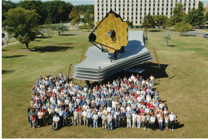
Plate 19 A full-scale model of the James Webb Space Telescope (JWST), the successor to the Hubble Space Telescope ( http://www.jwst.nasa.gov/ ; see Figure 10.2 and associated discussion for more information). JWST includes a primary mirror 6.5 m in diameter and offers instrument sensitivity across the IR wavelength range of 0.6 to 28\ \mu\text{m} , which will allow detection of the first generations of galaxies. The size of the Sun shield (the large flat screen in the image) is 22 m \times 10 m (72 ft \times 29 ft). The telescope will orbit 1.5 million km from Earth at the Lagrange L2 point. Courtesy of NASA/EPO.
