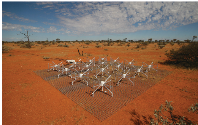
Plate 30 One of the antenna “tiles” used in the Murchison Widefield Array (MWA) experiment in Western Australia (see Figure 12.19 and associated discussion for more information). Each such tile is composed of 16 crossed-dipole antennae, with their signals combined through hardware at the station. The full telescope combines the signals from \sim 128 tiles interferometrically. This allows for a large (several hundred square degree) field of view with a moderately large collecting area. The antennas operate in the range 80–300 MHz, corresponding to z \approx 6 –15 (although the telescope will be sensitive to the spin-flip background only at z < 10 ). C. Lonsdale.
