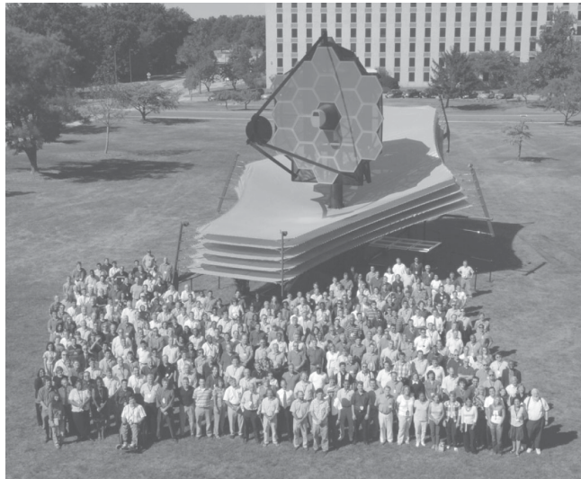
Figure 6.4. A full-scale model of the James Webb Space Telescope (JWST), the successor to the Hubble Space Telescope ( http://www.jwst.nasa.gov/ ). JWST includes a primary mirror 6.5 meters in diameter, and offers instrument sensitivity across the infrared wavelength range of 0.6\text{--}28\ \mu\text{m} which will allow detection of the first galaxies. The size of the Sun shield (the large flat screen in the image) is 22 meters \times 10 meters (72 ft \times 29 ft). The telescope will orbit 1.5 million kilometers from Earth at the Lagrange L2 point.
