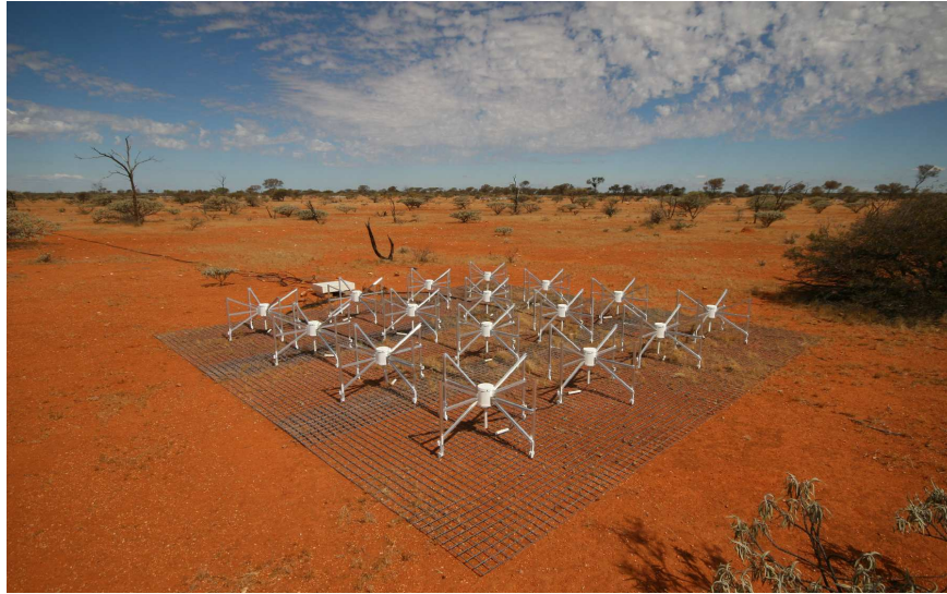
Figure 11.17 One of the antenna “tiles” used in the Murchison Widefield Array (MWA) experiment in Western Australia. Each such tile is composed of 16 crossed-dipole antennae, with their signals combined through hardware at the station. The full telescope combines the signals from the 500 tiles interferometrically. This allows for a large (several hundred square degree) field of view with a moderately large collecting area \sim 8,000 \text{ m}^2 (comparable to the Very Large Array). The antennae operate between 80–300 MHz, corresponding to z \approx 6 –15 (although the telescope will only be sensitive to the spin-flip background at z < 12 ). Image credit: C. Lonsdale.
