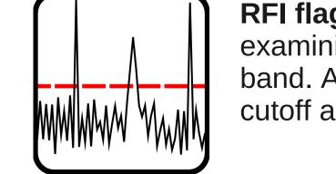
**RFI flagging.** High-duty-cycle RFI is flagged by examining the summation of *all* of the data in a given band. Amplitude spikes above an interactively-specified cutoff are considered RFI and flagged as bad.
