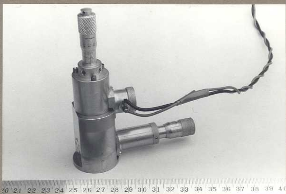
Figure 2.6 (a): A fully assembled Gunn oscillator.
